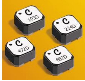
Figure 1.4. LPD 5030V series miniature high-isolation 1:1 two-winding inductor with 1500 V isolation voltage at least occupy 5 \times 5 \text{ mm}^2 footprint and 2.9 mm thickness for an inductance of 4.7 \text{ }\mu\text{H} [6].
